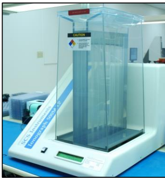
Ionograph Cleanliness Testing
